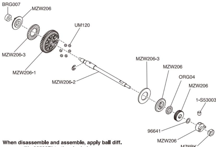
When disassemble and assemble, apply ball diff.
